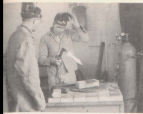
R. Townsend and G. Wirth using "oxy-" acetylene cutting torch.
